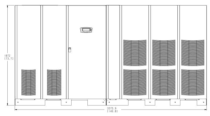
Figure 3-1. UPS Cabinet Dimensions (Front View)
